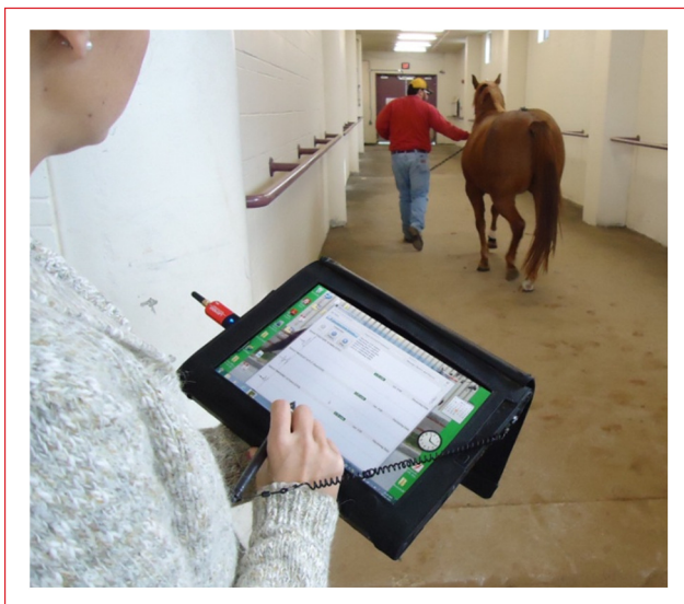
Bluetooth technology captures data from the Lameness Locator sensors and transfers the information to a wireless tablet with software that produces a computer readout with the data results
