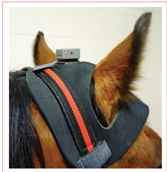
The Lameness Locator consists of three rechargeable electronic sensors, two of which are accelerators that are placed on the horse's head and pelvis, and the third is a gyroscope that is situated on the horse's right foreleg
