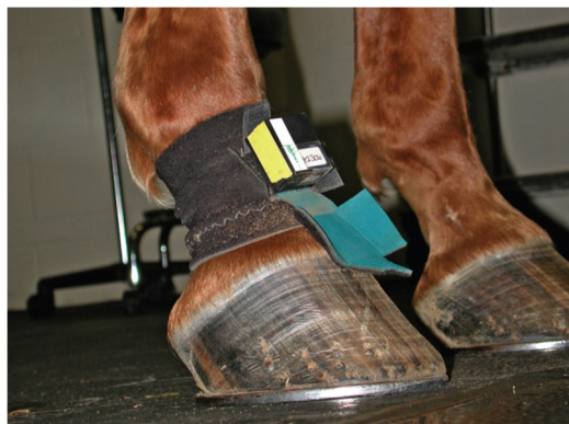
The Lameness Locator evaluates soundness based on the vertical motion of the torso, so the gyroscope placed on the horse’s right foreleg should have no bearing on how the horse’s torso accelerates and
